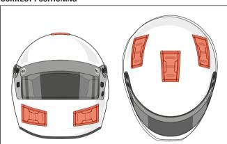
Before installing the Cover Plate, remove the protective cover from the back side of the Cover Plate exposing the adhesive material that will seal the Cover Plate to the helmet shell. Once installed press firmly around the edges of the Cover Plate to assure proper adhesion.
