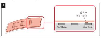
Place the Forced Air and Cover Plate Seals on top of the Cover Plate to ensure a perfect seal and prevent air from entering (illustration 02).
